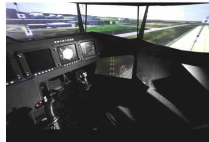
Figure 3. Inside the Piloting Cab of the Vertical Motion Simulator (VMS).
