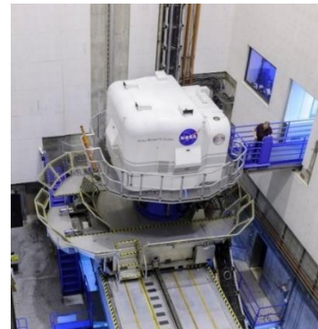
Figure 2. Vertical Motion Simulator (VMS) Cab and Actuator System Located at NASA Ames (Ref. 8).
