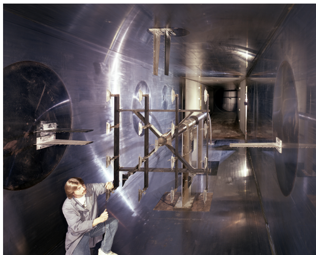
Fig. 6 17-Wedge Array installed in the 10x10 SWT test section during the 1991 test section characterization test entry. GRC-1991-C-09146.
