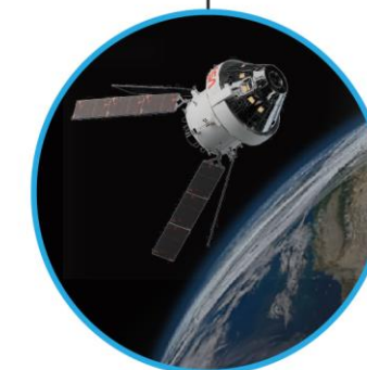
O2O Orion Artemis II Optical Communications System 260 Mbps downlink 20 Mbps uplink Lunar-to-Earth
