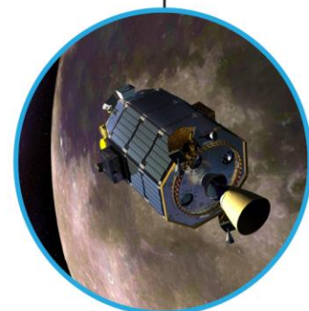
LLCD Lunar Laser Communications Demonstration 622 Mbps downlink 20 Mbps uplink Lunar-to-Earth
