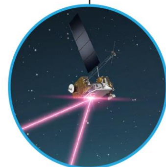
LCRD Laser Communications Relay Demonstration 1.2 Gbps downlink 1.2 Gbps uplink GEO-to-Earth and GEO-to-LEO
