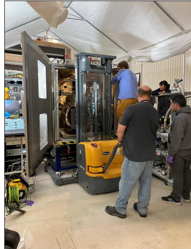
Loading reactor into ASSSIT chamber
