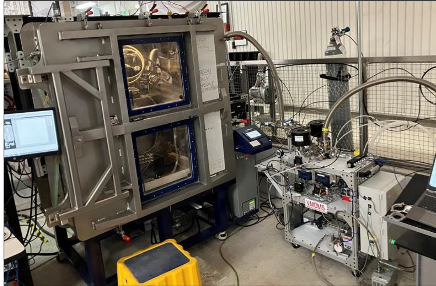
LR-1 in ASSIST under vacuum pressure (Front Deflector Shield excluded during this pump-down). System reached 9.84\text{E}-06 Torr on ASSIST and 0.8 torr on LR-1 during leak checks.
