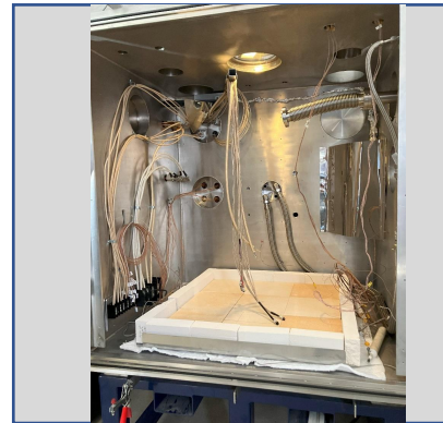
ASSIST Environment Chamber Outfitted for Reactor Integration
