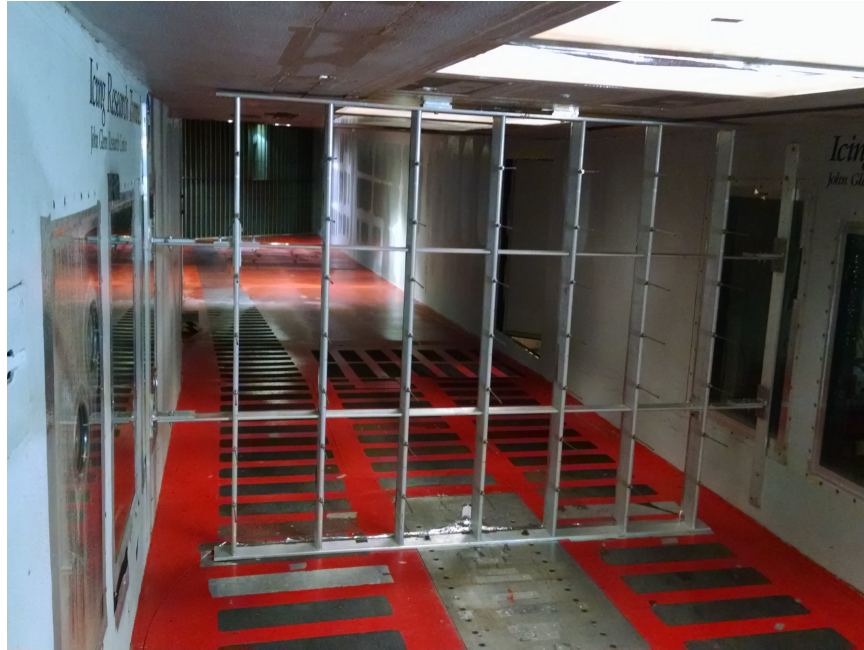
Figure 6. 2D RTD array mounted in the IRT test section (forward looking aft).
