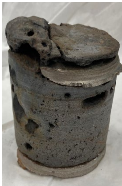
Figure 1. Core sample removed from reactor after MRE testing complete.
