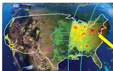
(A) Aerial view of TEMPO coverage across North America, mapping high-resolution measurements hourly. (B) Spatial coverage of TEMPO pixels over several days at 12:00 with reference Pandora Station 40 in Washington DC (38.9218, -77.0124) in January 2025. Spatial resolution is consistent over ground sensor, ensuring continuous coverage for evaluation.
