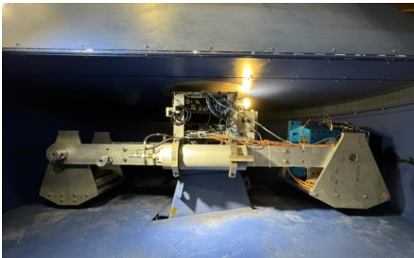
Fig 5. SRSC #4 configured for 6.3g lateral 2 testing on 2023-12-13.
