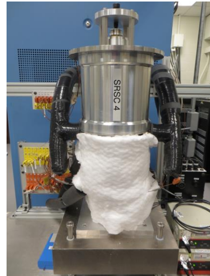
Fig. 8. SRSC #4 on test stand with thermal cycling hardware installed.
