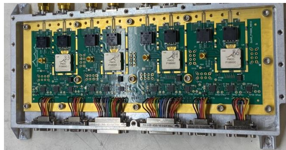
Quad-ASIC board for CoSMIR-H
