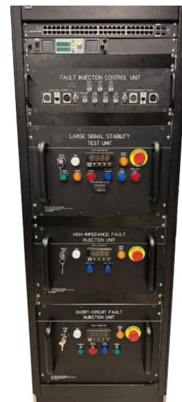
Fig. 1. DC Fault Injection Unit
