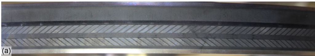
Figure 39.—NCFS Build 2 room-temperature dynamic test wear results. (a) Prior to lift-off test. (b) After lift-off test. (c) After performance test at 69 kPa pressure differential.
