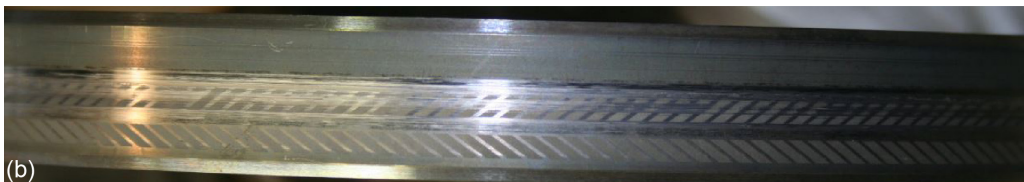
Figure 40.—Herringbone-grooved rotor used with NCFS Build 2. (a) Prior to static and dynamic performance tests. (b) After room-temperature performance test at 69 kPa pressure differential.
