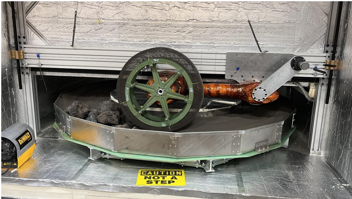
Figure 19. EXtreme Terrain Endurance Rig (XTERra) at NASA GRC shown with a bin of JSC-1A and volcanic rocks.
