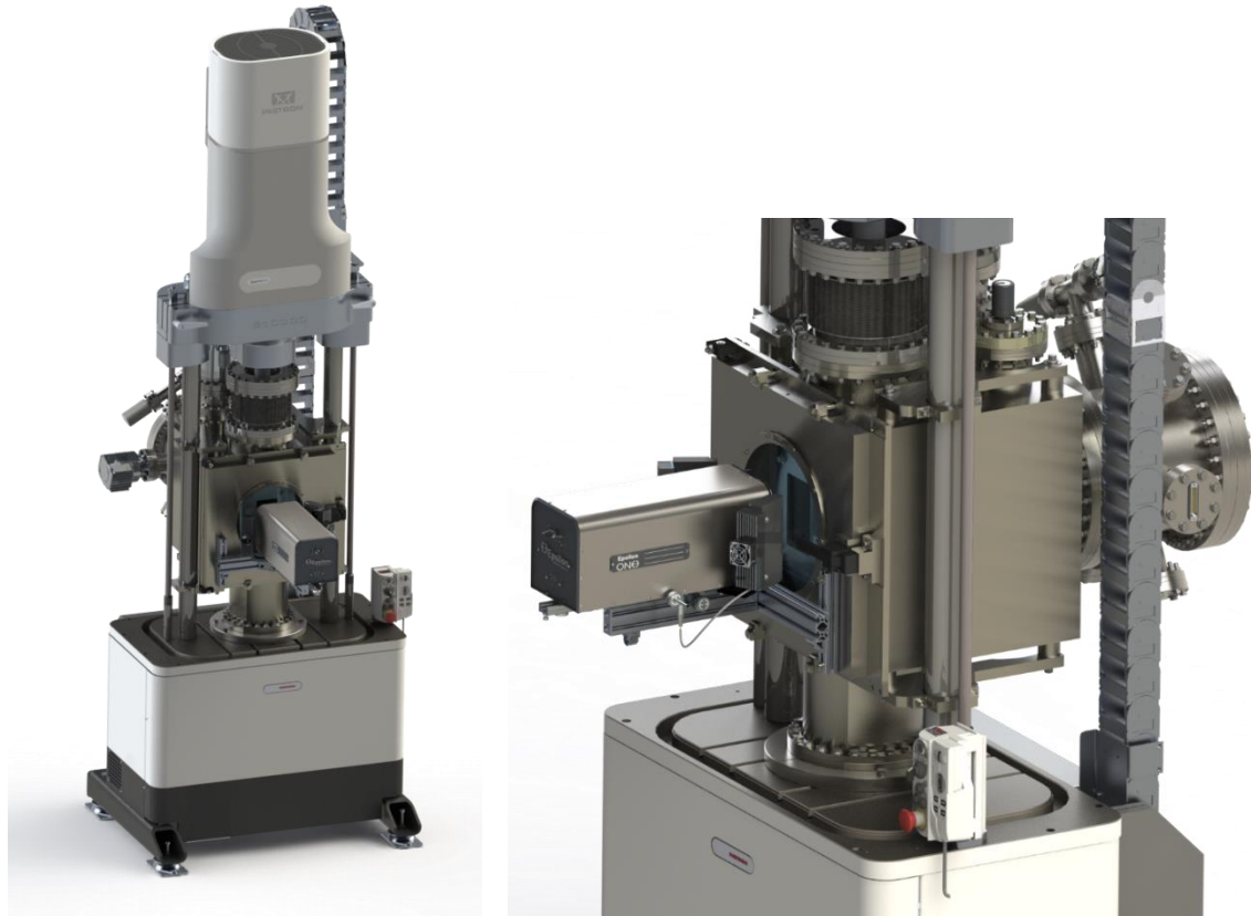
Figure 16. Design concept for the Lunar Environment Strength Test Rig at NASA GRC.
