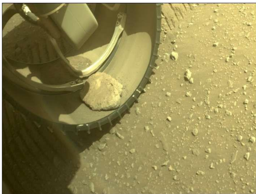
Figure 21. Photo of Mar's Perseverance rover with rock stuck in one of the wheels (credit NASA/JPL-Caltech).
