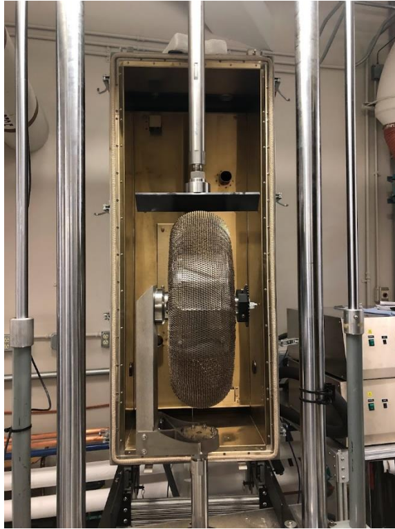
Figure 17. EXtreme Cyclic Environmental Load (XCEL) test rig at NASA GRC.
