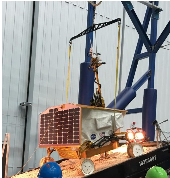
Figure 26: Resource Prospection Rover in ARGOS
