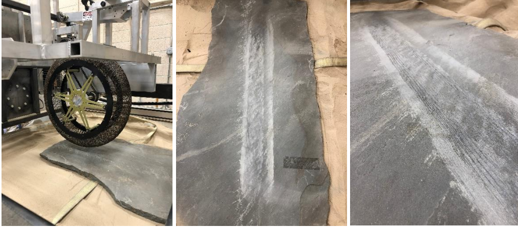
Figure 22. NASA GRC Mars Spring Tire prototype in friction testing setup (left) along with resulting abrasion created on the bedrock surface (center and right image).
