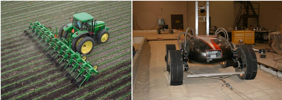
Figure 1: (a) Farming tractor towing a drawbar load. (b) Roving vehicle undergoing drawbar pull testing
