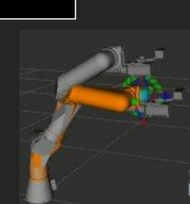
Robotic laser welder in simulated environment as digital twin of actual process
