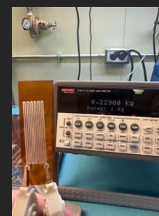
Strain Sensor Test Specimens printed at MSFC
