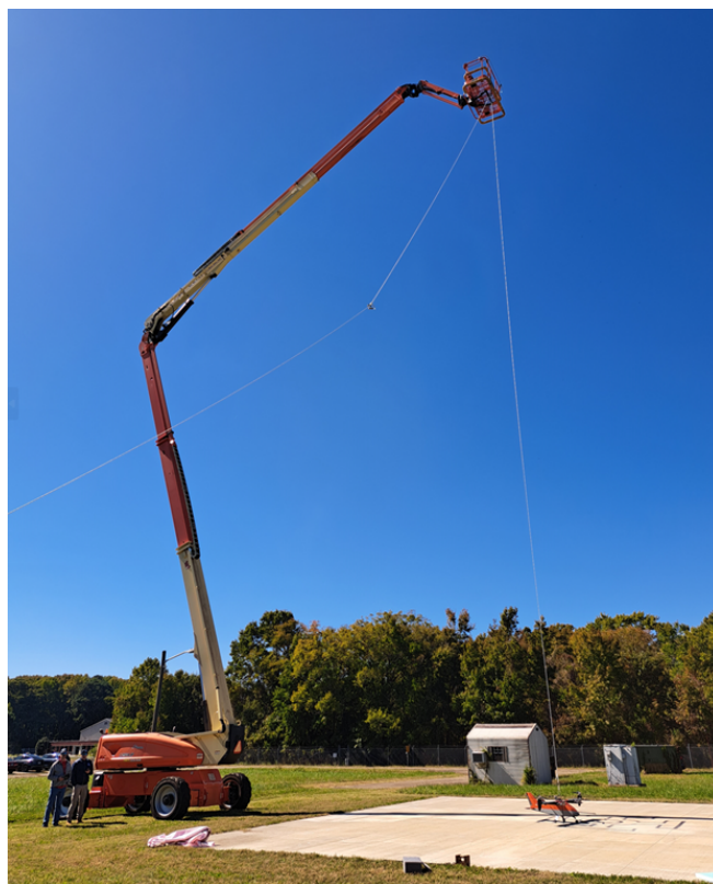
Figure 15: RAVEN-SWFT tethered flight-test setup.
