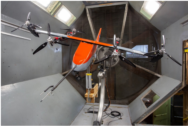
Figure 3: RAVEN-SWFT mounted on a 3DOF free motion wind-tunnel apparatus in the NASA LaRC 12-Foot LST. (Credit: NASA)
