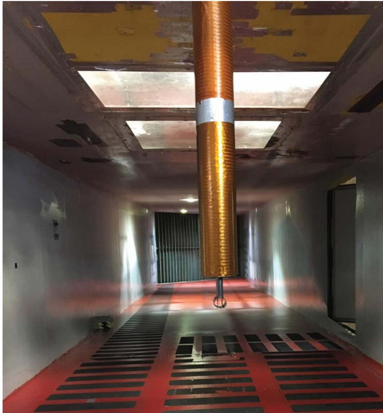
Figure 12.—Multi-Element Sensor (Science Engineering Associates, Inc.) mounted in the test section.
