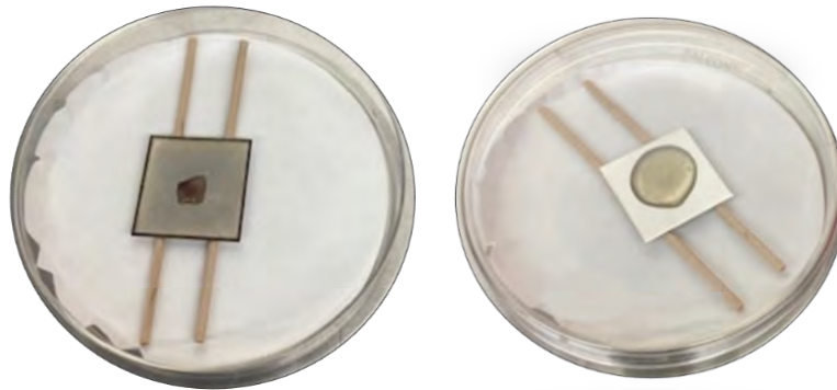
Figure 71.—Closeup of two coupons configured for microbial testing (Ref. 12).
