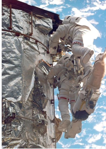
Figure 1. Large cracks in the outer layer of solar facing MLI on the HST as observed during SM2 after 6.8 years of space exposure. 6
