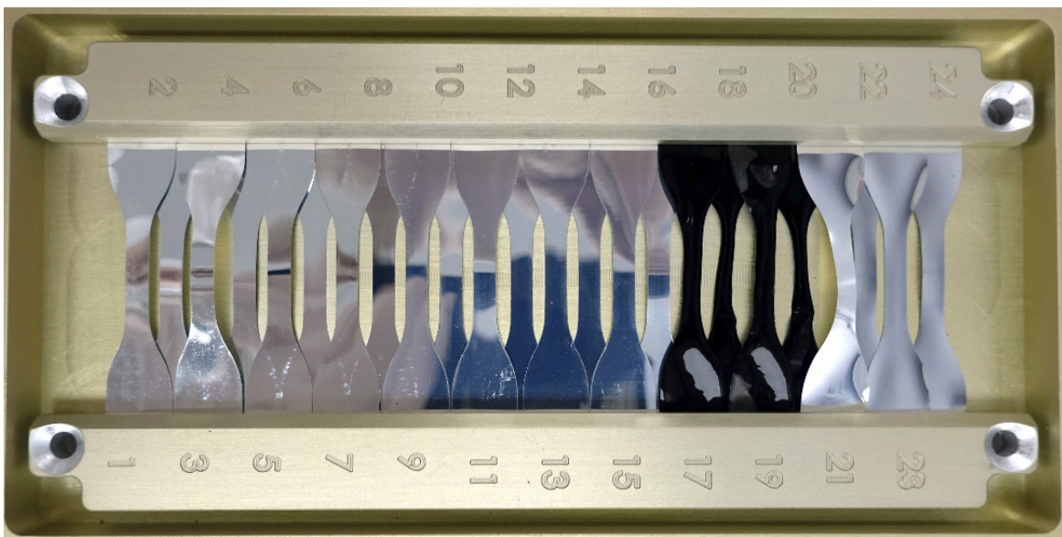
Figure 26. Post-flight photograph of the MISSE-9 PCE-1 zenith tensile samples.
