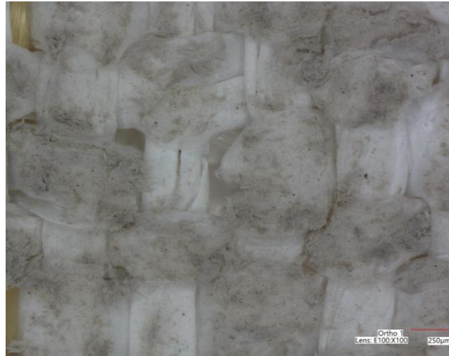
Figure 4. Dust Covered Ortho Fabric Tumbler Panel (Top), Dust Covered and Abraded Ortho Fabric at 100x (Bottom). Dust coats the face side of the Ortho Fabric after tumbling darkening its color. The abrasion has caused the Gore-Tex® fibers to tuft and discolor.
