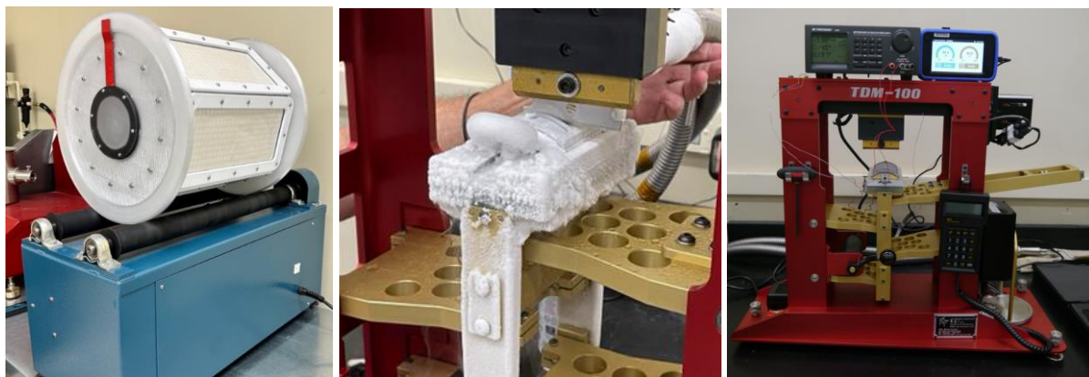
Figure 2. Rotary Abrasion Tumbler (Left), Cryo Cut Resistance Test (Center), Hot Cut Resistance Test (Right). These tests are designed to condition fabrics with abrasion caused by rock and dust as well as temperature extremes to study the fabrics durability.
