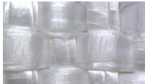
Figure 1. Beta Cloth (Top) and Ortho Fabric (Bottom). Beta Cloth was a single layer fabric made from Beta fibers coated with Teflon. Ortho Fabric is a double layer cloth with a face side composed of Gore-Tex slit film yarn.
