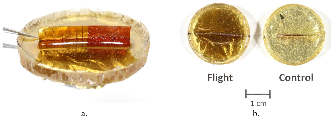
Figure 35. Post-flight photographs of the Au-Kapton H/Epoxy sample (M10Z-C10 F): a). Image of the flight sample showing the \frac{1}{2} scratched Au coated surface and the \frac{1}{2} NaCl sprayed surface, and b). Visible light image of the flight (F) and control (B) samples.
