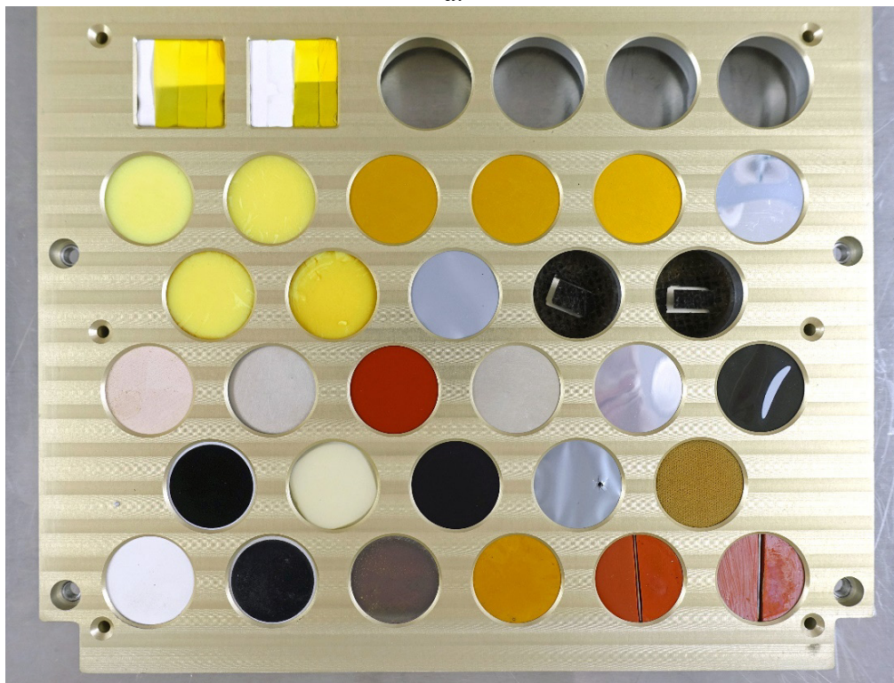
Figure 39. Photographs of the MISSE-12 PCE-3 ram SS deck (R2 MSC 4): a). Pre-flight with the PCE-3 ram samples, and b). Post-flight showing discoloration of the MSC deck and numerous samples.
