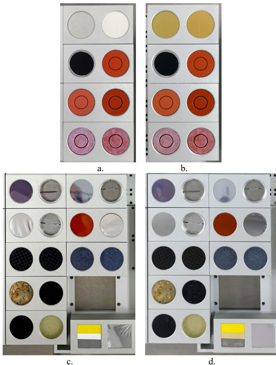
Figure 56. Photographs of the MISSE-13 PCE-4 wake MS deck (W1 MSC 5): a). Pre-flight of the upper deck samples, b). Post-flight of the upper deck samples, c). Pre-flight of the lower deck samples, and d). Post-flight of the lower deck samples.
