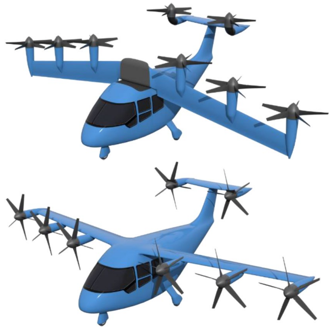
Figure 1. Renderings of the Tiltwing reference model in hover (top) and cruise (bottom) configurations (Ref. 5).
