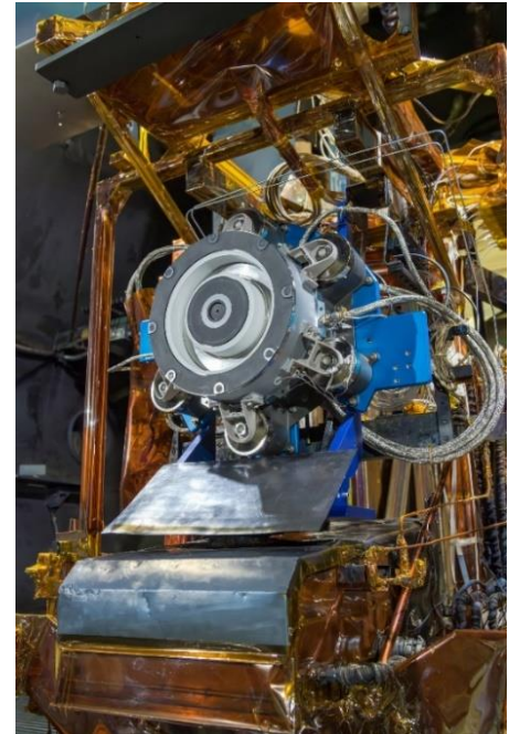
Fig. 5 AEPS QM1 installed at VF-5 at NASA GRC
