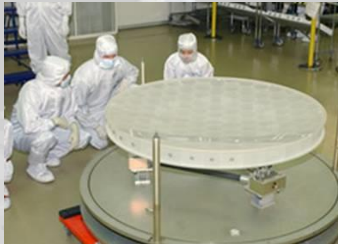
1.5 Meter Primary Mirror for Kepler Spacecraft Image courtesy NASA/JPL
