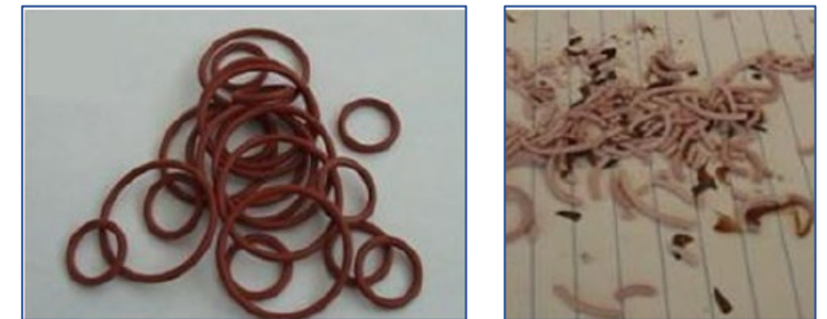
O-ring radiation damage [4]
