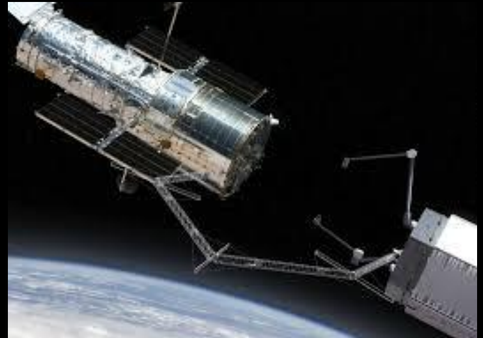
Tendon-Actuated Lightweight In-Space MANipulator (TALISMAN)
