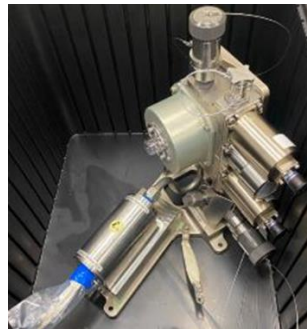
Figure 5. UWMS spare dosing assembly.
