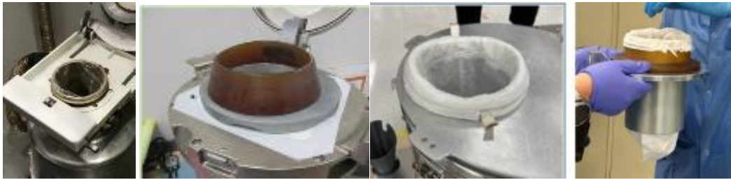
Figure 8. a) Russian WHC use with fecal bag, b) Orion UWMS with original 5" seat and original UWMS fecal bag installed, c) LOO seat design with fecal bag installed, d) Updated seat with updated fecal bag (design #2).
