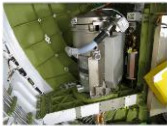
Figure 1. Orion UWMS installed in Artemis-II vehicle.
