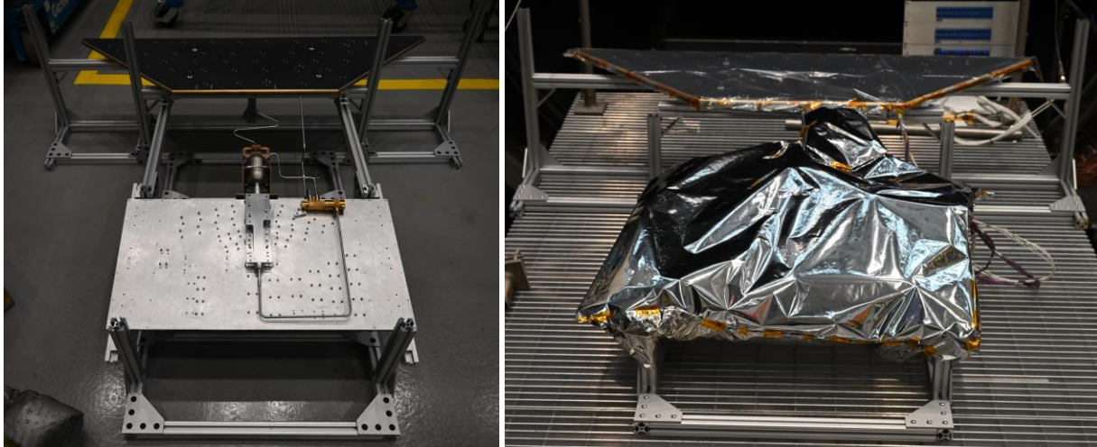
Figure 3. Left: top view of the TMS test article without MLI. Right: TMS test article with MLI.
