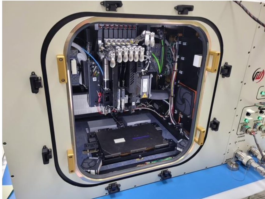
Figure 2: FabLab – Printer Module with Advanced Toolplate Engineering Development Unit (EDU) (Credit: Redwire Space Technologies).
