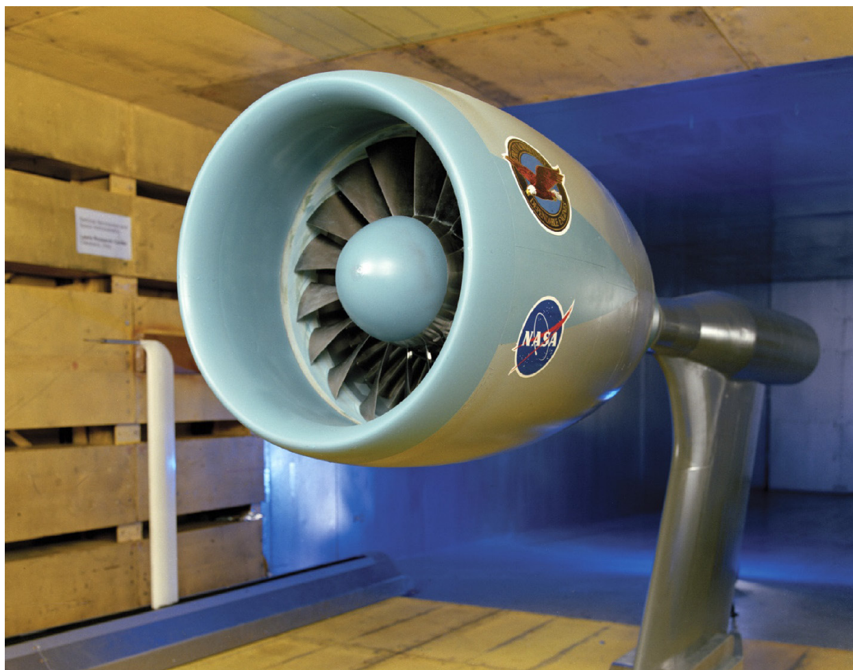
Figure 1.—Advanced Ducted Propulsor fan test in 1995 (NASA Image C-1995-1896).
