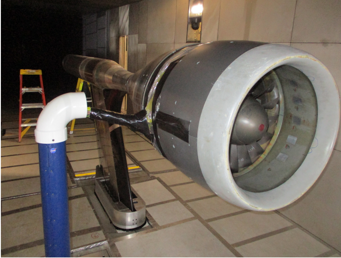
Figure 20.—Instrument tube used as cable run for taking wires and tubes off outer duct.
