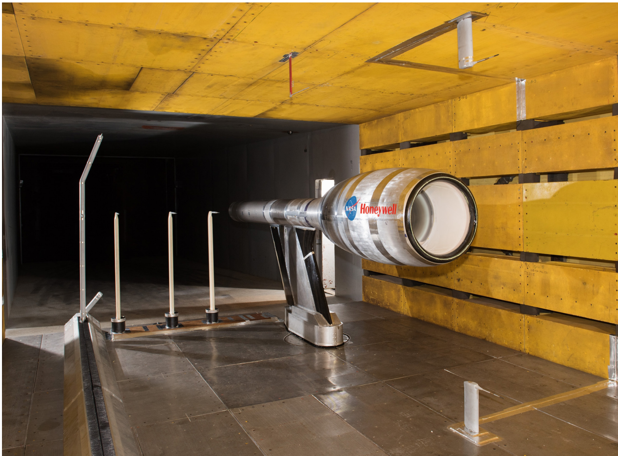
Figure 15.—Microphone layout used for 2014 Honeywell test.
