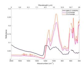
Example comparison of a slice, shocked to 10 GPa. C1a and C1b are front and back of the pre-shock slices. **References:**
