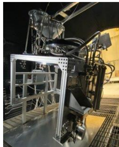
Fig. 7. Back Side of the Carbothermal Reactor inside NASA JSC's B351 Dirty Thermal Vacuum Chamber.
