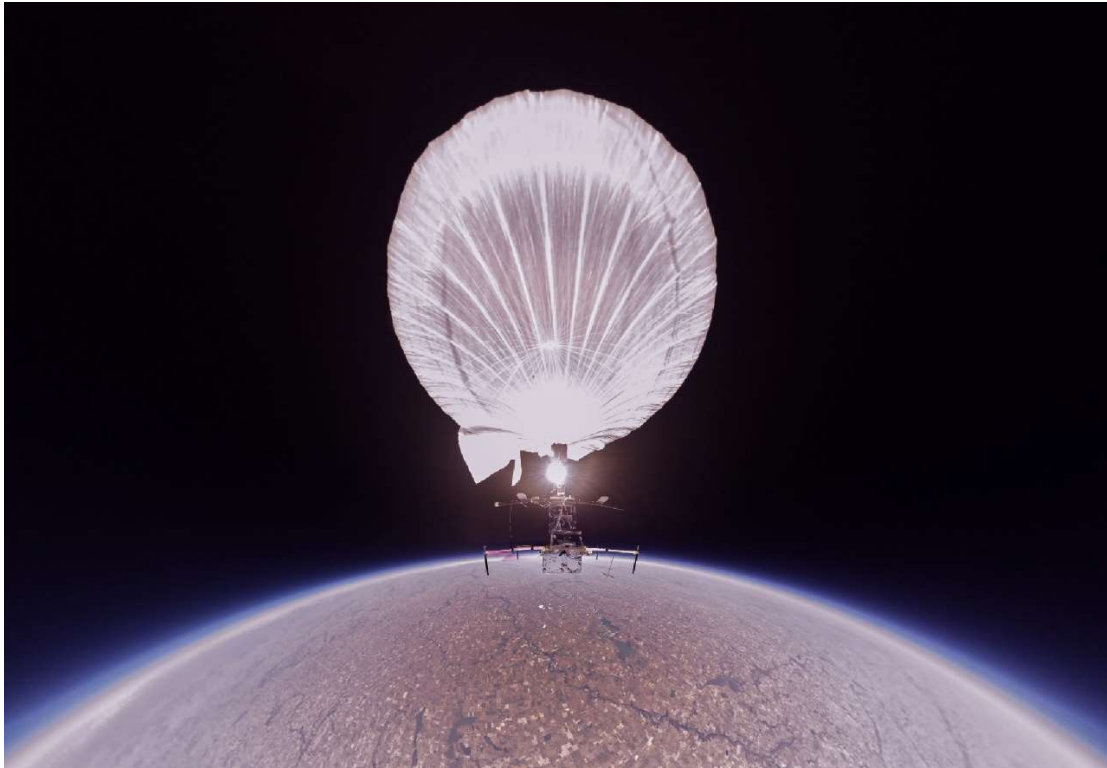
Figure 6: The FIGARO Flight Communications Payload flying aboard an Aerostar Cyclone balloon floating at an altitude of 30 km.
