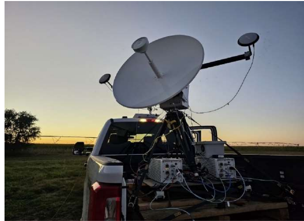
Figure 4: The Wideband Terminal mounted into the back of a 4x4 pick-up truck on preparation for flight demonstration.
