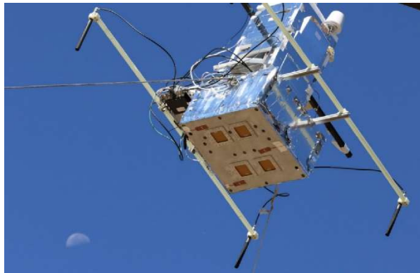
Figure 3: The FIGARO Flight Payload Transponder attached to Aerostar's Flight Control Unit.
