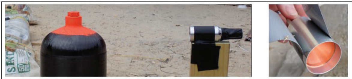
Figure 44: Test 6 Conical Shaped Charge Setup (L) and Standalone Picture (R)
