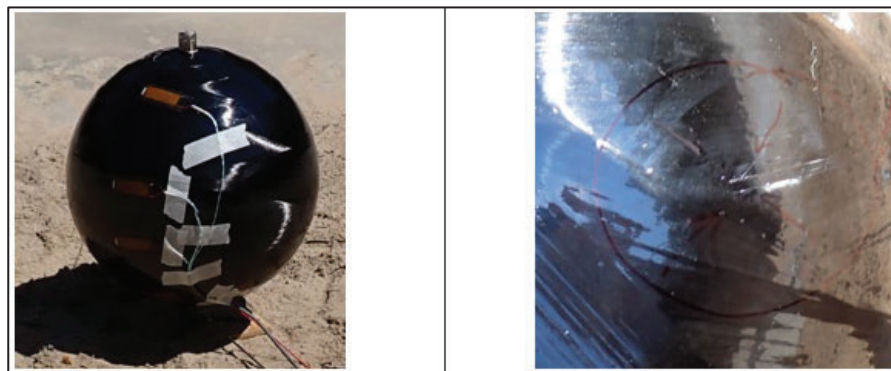
Figure 94: Test 21 Cimarron Tank Pre-Test (L) and Post-Test Stress Cracks (R)
