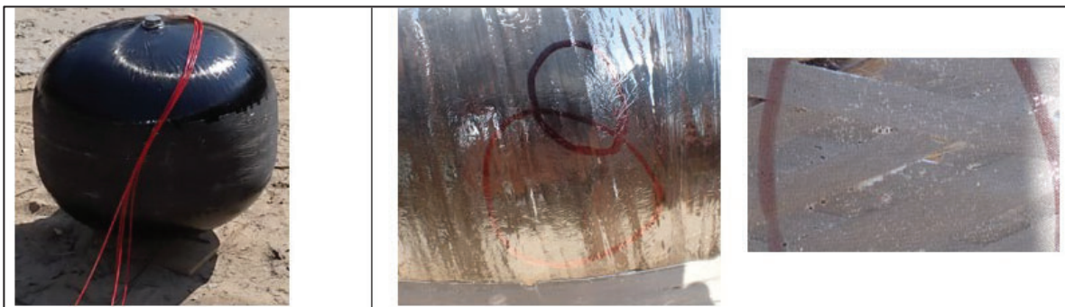
Figure 98: Test 22 HyPerComp Tank Pre-Test (L) and Post-Test Stress Cracks (C)(R)
