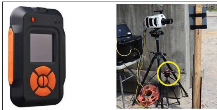
Figure 16: MIOPS Acoustic Trigger System (L), and Implementation (R)
