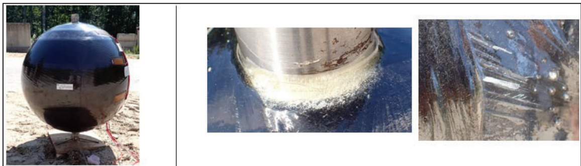
Figure 92: Test 18 Cimarron Tank Pre-Test (L) and Post-Test Stress Cracks (R)
