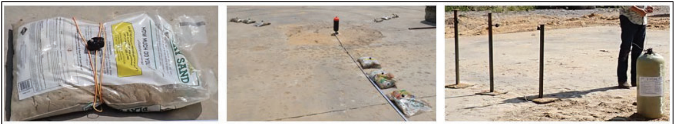
Figure 18: BOP Sensor Implementation Methods: Mounted to Sandbag (L), BOP Sensor Array (C), Mounted to Poles (R)
