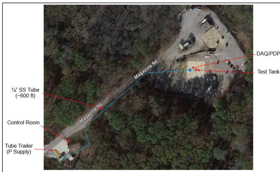
Figure 4: Schematic of COPV N 2 Fill System
