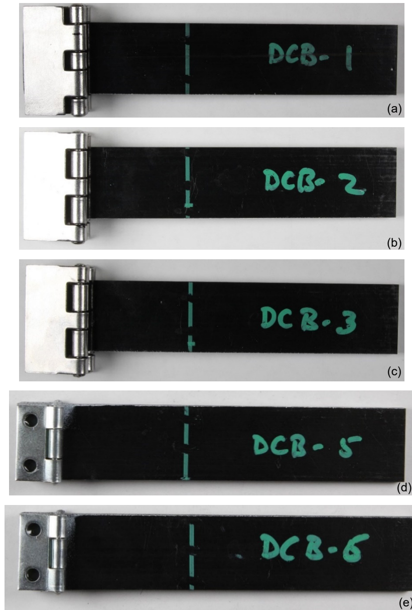
Figure 85.—DCB specimens prior to testing. (a) HUDC_DCB-1. (b) HUDC_DCB-2. (c) HUDC_DCB-3. (d) HUDC_DCB-5. (e) HUDC_DCB-6.
