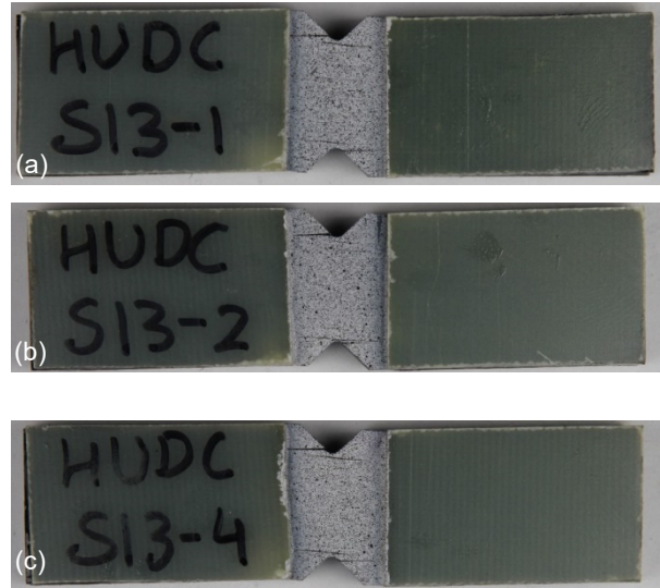
Figure 65.—1-3 plane shear specimens after testing. (a) HUDC_S13-1. (b) HUDC_S13-2. (c) HUDC_S13-4.
