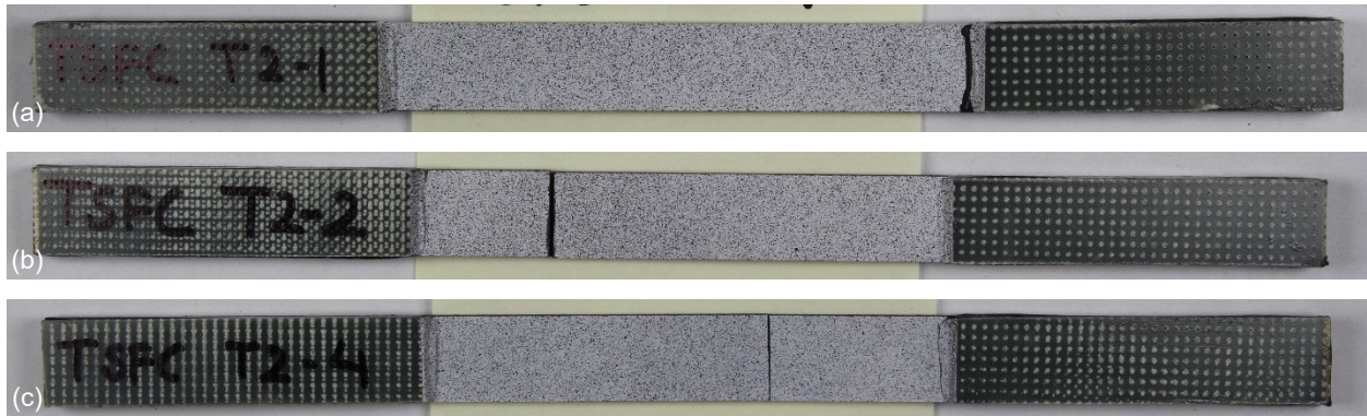
Figure 16.—2-direction tension specimens after testing. (a) TSFC_T2-1. (b) TSFC_T2-2. (c) TSFC_T2-4.
