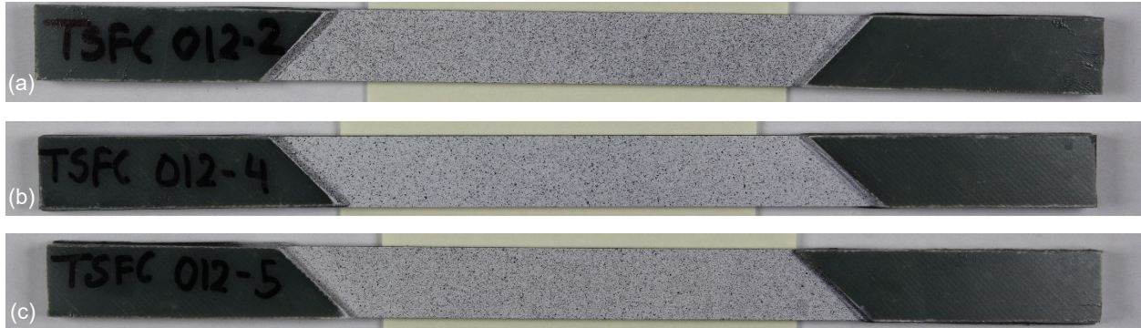
Figure 74.—1-2 plane 45° off-axis tension specimens prior to testing. (a) TSFC_O12-2. (b) TSFC_O12-4. (c) TSFC_O12-5.
