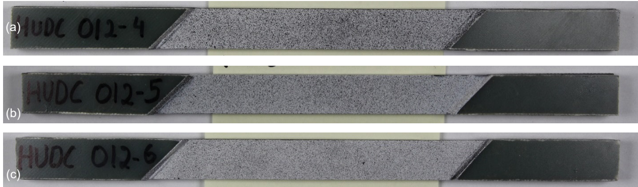
Figure 71.—1-2 plane 45° off-axis tension specimens prior to testing. (a) HUDC_O12-4. (b) HUDC_O12-5. (c) HUDC_O12-6.
