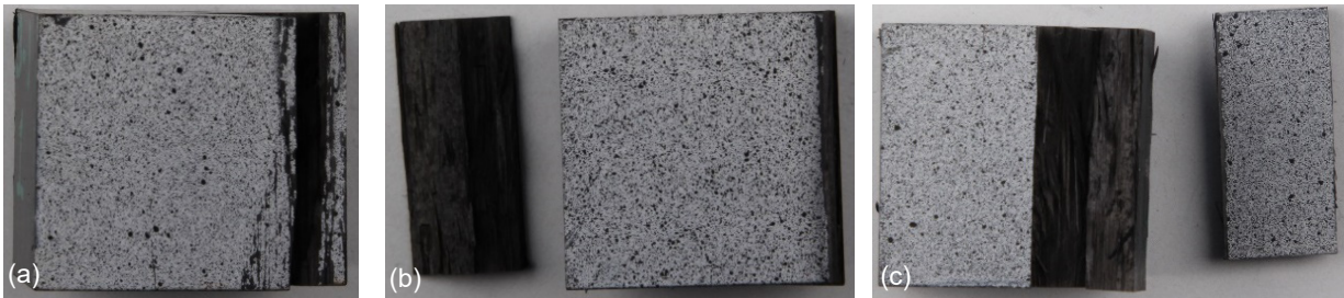
Figure 42.—3-direction compression specimens after testing. (a) HUDC_C3-1. (b) HUDC_C3-2. (c) HUDC_C3-3.
