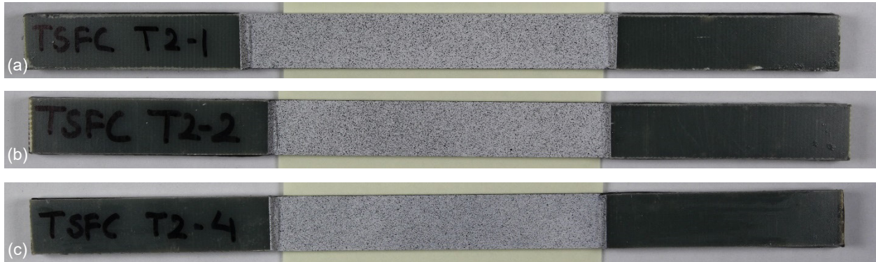
Figure 15.—2-direction tension specimens before testing. (a) TSFC_T2-1. (b) TSFC_T2-2. (c) TSFC_T2-4.
