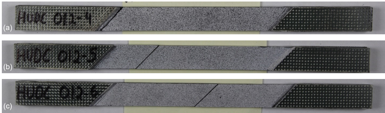
Figure 72.—1-2 plane 45° off-axis tension specimens after testing. (a) HUDC_O12-4. (b) HUDC_O12-5. (c) HUDC_O12-6.
