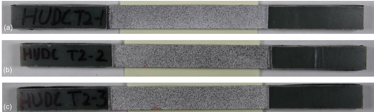
Figure 12.—2-direction tension specimens before testing. (a) HUDC_T2-1. (b) HUDC_T2-2. (c) HUDC_T2-3.
