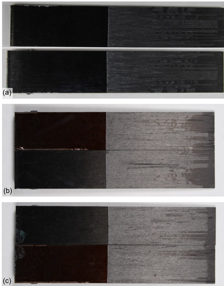
Figure 90.—DCB specimens after testing. (a) TSFC_DCB-2. (b) TSFC_DCB-4. (c) TSFC_DCB-6.
