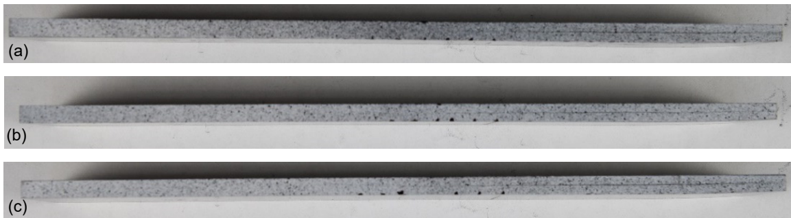
Figure 98.—ENF specimen after testing. (a) TSFC_ENF-1. (b) TSFC_ENF-2. (c) TSFC_ENF-3.
