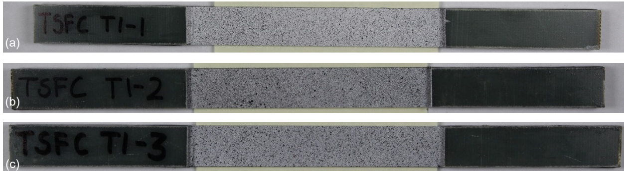
Figure 8.—1-direction tension specimens before testing. (a) TSFC_T1-1. (b) TSFC_T1-2. (c) TSFC_T1-3.
