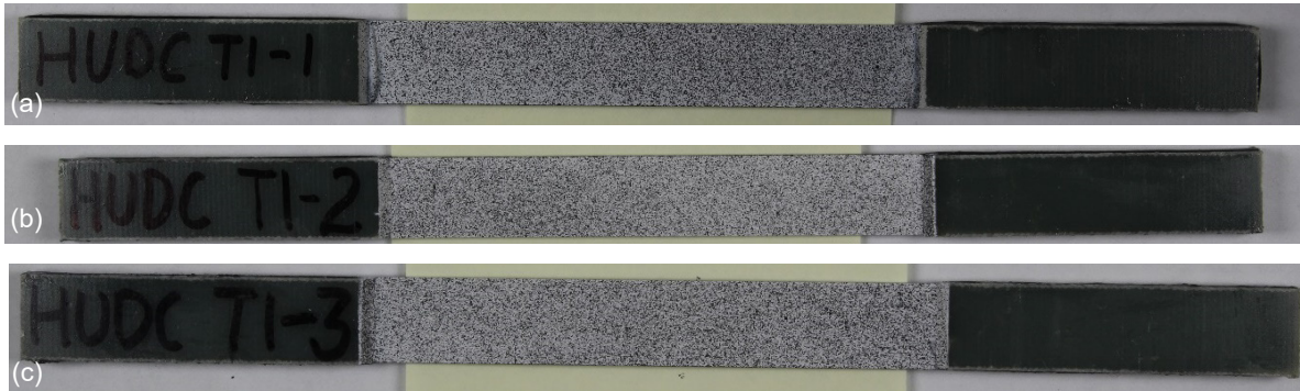
Figure 5.—1-direction tension specimens before testing. (a) HUDC_T1-1. (b) HUDC_T1-2. (c) HUDC_T1-3.
