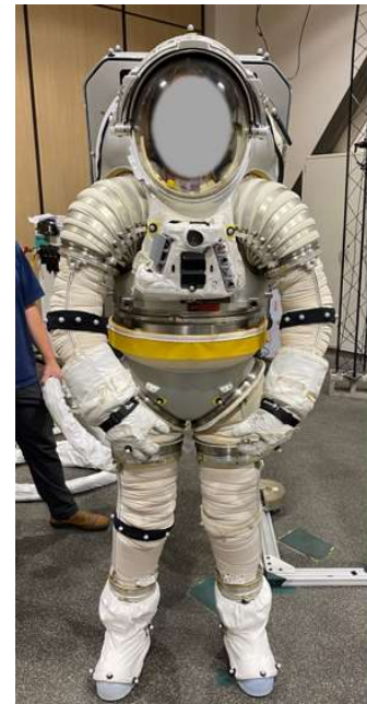
Figure 1. Optical Motion Capture markers Placed Across the xEMU Spacesuit.
