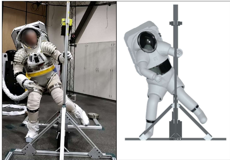
Figure 4. Example of xEMU Spacesuit HITL Data Extrapolated to a 99 th Percentile Human-Suit Model Using Motion Capture Kinematics Data. The suited subject is performing a side-squat-step technique to translate through a simulated hatch.
