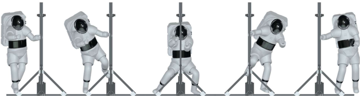
Figure 7. 99 th Percentile resized xEMU Human-suit model transitioning through a 60x40-inch Hatch, with a 12-inch step threshold. Kinematic data captured from xEMU spacesuit hatch evaluation test series were used to create a dynamic human-suit model.
