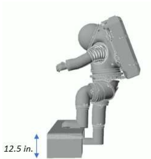
Figure 5. 1 st Percentile resized xEMU Human-suit model Performing a Step Up. Kinematic data captured from xEMU DVT series used to create a static step-up posture.
