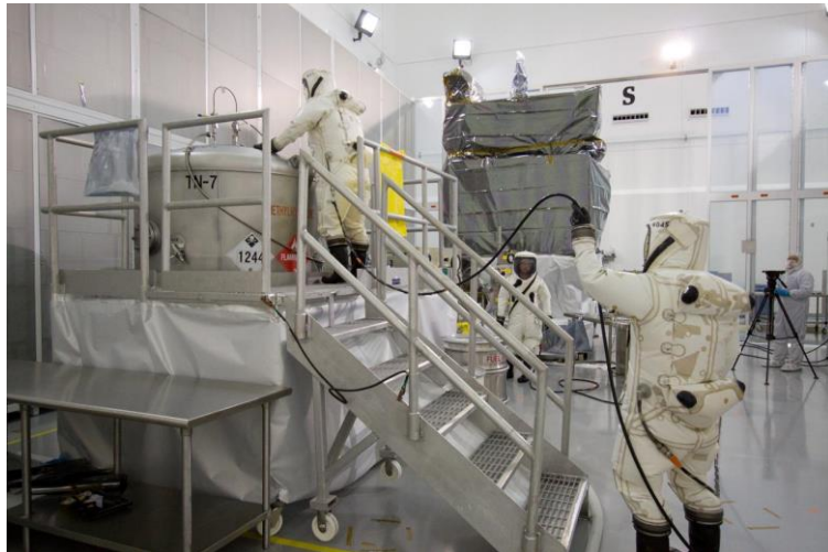
Spacecraft fueling technicians from Kennedy Space Center take a sample of the monomethylhydrazine propellant
