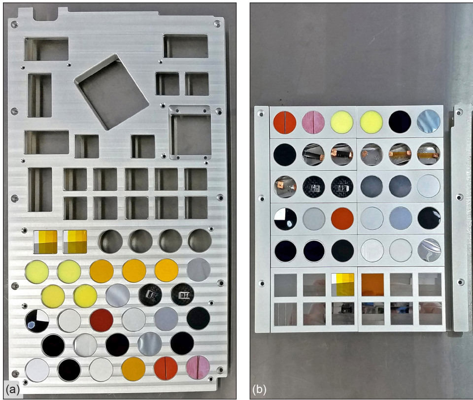
Figure 10.—Carrier trays preflight with MISSE-12 test articles installed. (a) Ram. (b) Wake.
