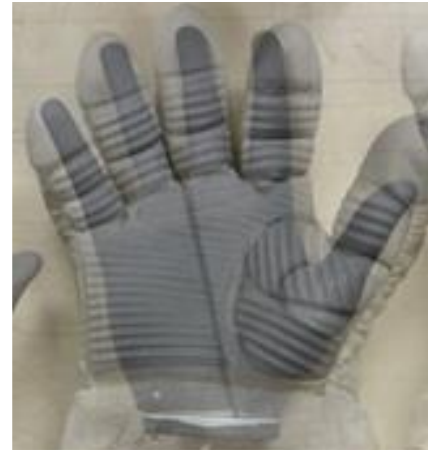
Figure 4. Hand form prototype overlay with EVA glove.
