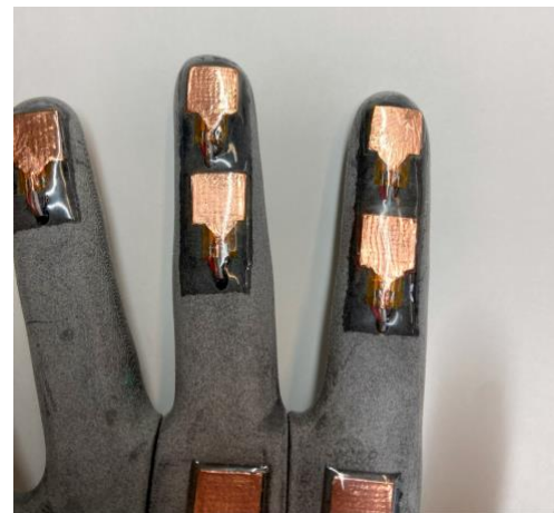
Figure 8. Surface sensors installed with protective layer.
