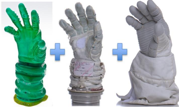
Figure 3. 3-Layer EVA glove assembly comprising the pressure bladder, thermal restraint layer and outer shell.
