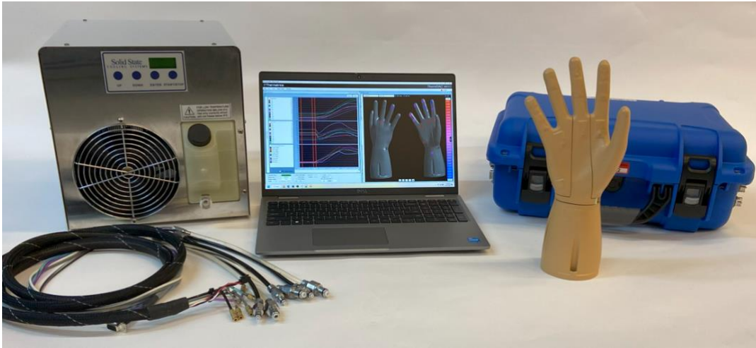
Figure 14. Completed hand manikin system, from left to right: Fluid + electrical harness, thermoelectric chiller, laptop with data acquisition software, thermal manikin device, portable control enclosure.
