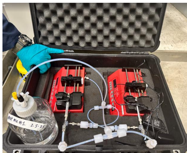
Figure 5. Injection pump system for liquid contaminants.
