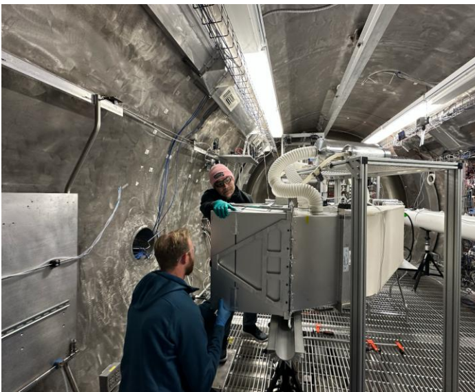
Figure 4. Pleated Filter Testbed Configuration at MSFC. Demonstrating simulated flight ingress operations.
