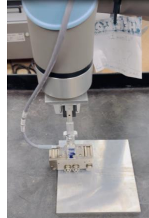
Non-contact, non-destructive robotic weld inspection
