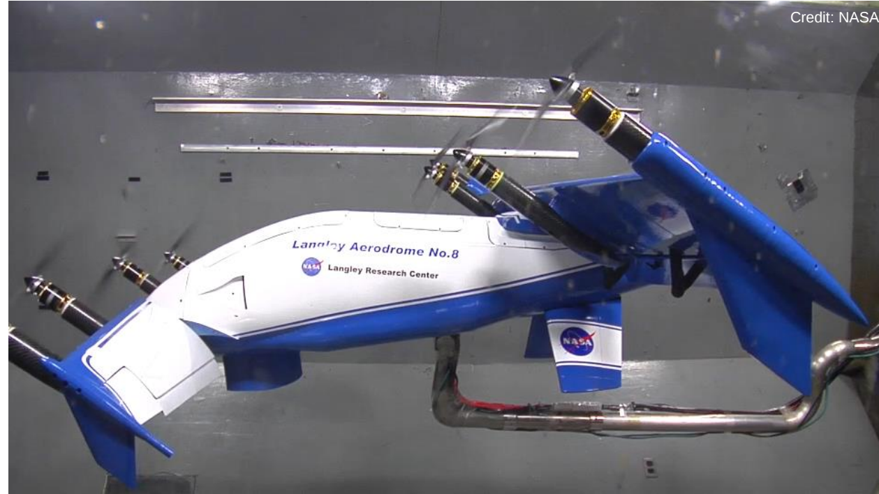
LA-8 DOE/RSM wind-tunnel testing.
