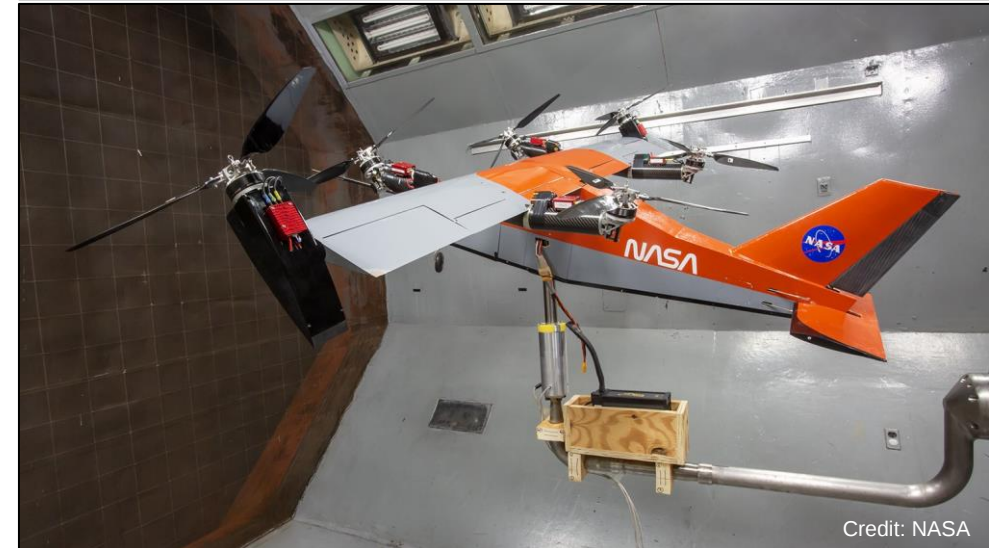
RAVEN-SWFT mounted on a 3DOF rig.
