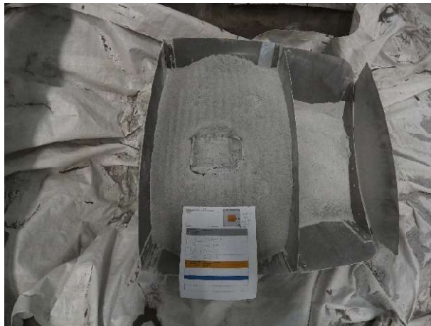
Figure 8. Trapezoidal LHS-1 bin within the BP-1 Big Bin after a spot compaction test.
