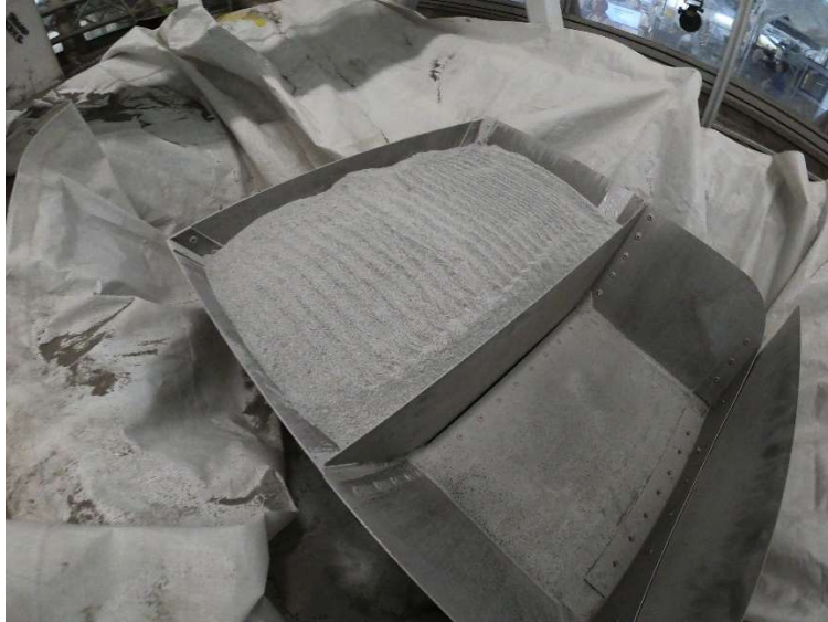
Figure 12. LHS-1 bin final raked surface before a compaction test begins.
