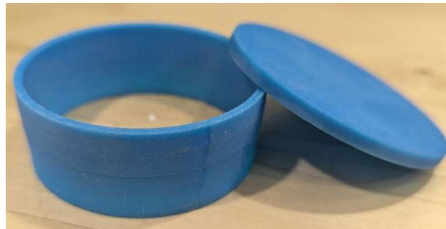
Figure 13. 60mm diameter 25 mm depth core sampler. Lid is used during transport to the scale and is installed prior to core excavation from the simulant surface.
