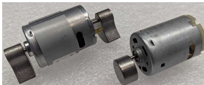
Figure 3. Dual-mass Z-Y motor (left) and single-mass X-Y motor (right).
