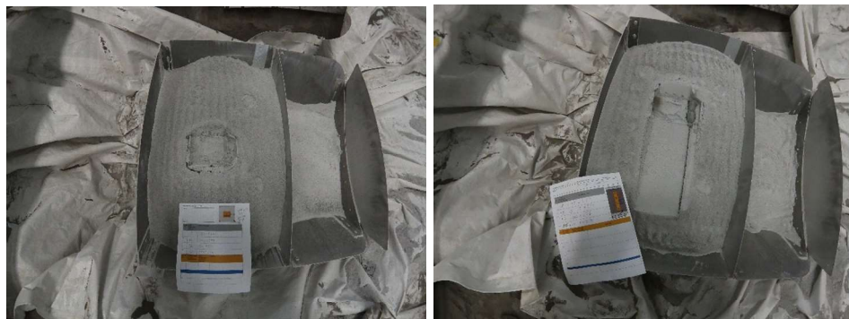
Figure 18. LHS-1 Spot (left) and Raster (right) compaction final test area surface.
