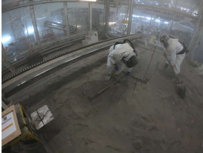
Figure 10. A pit is dug, and a previously excavated pit is covered by the 1 cm mesh screen and refilled with low density bulk regolith.
