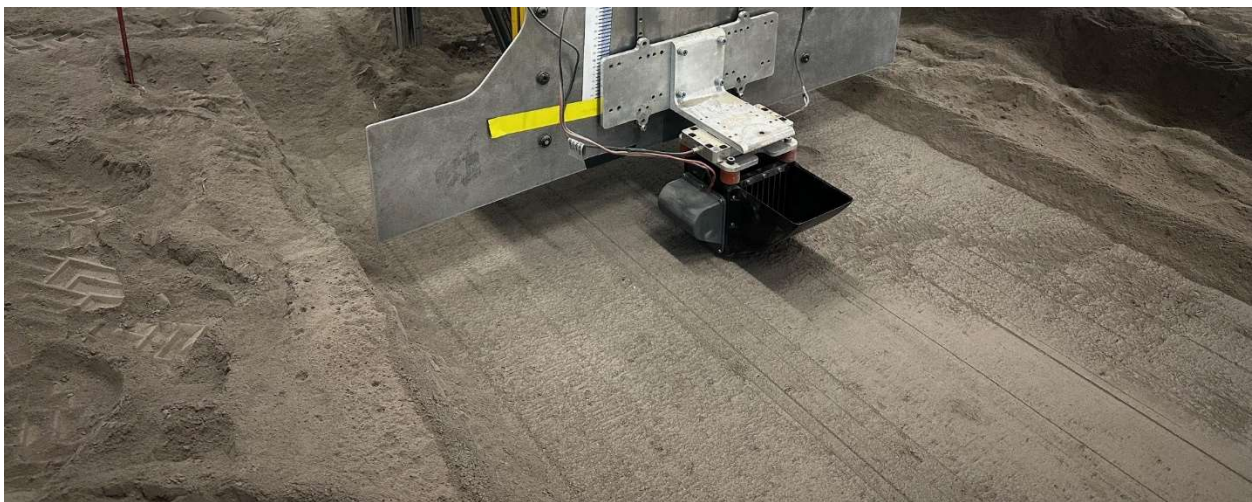
Figure 11. BP-1 surface after preparation and leveling.
