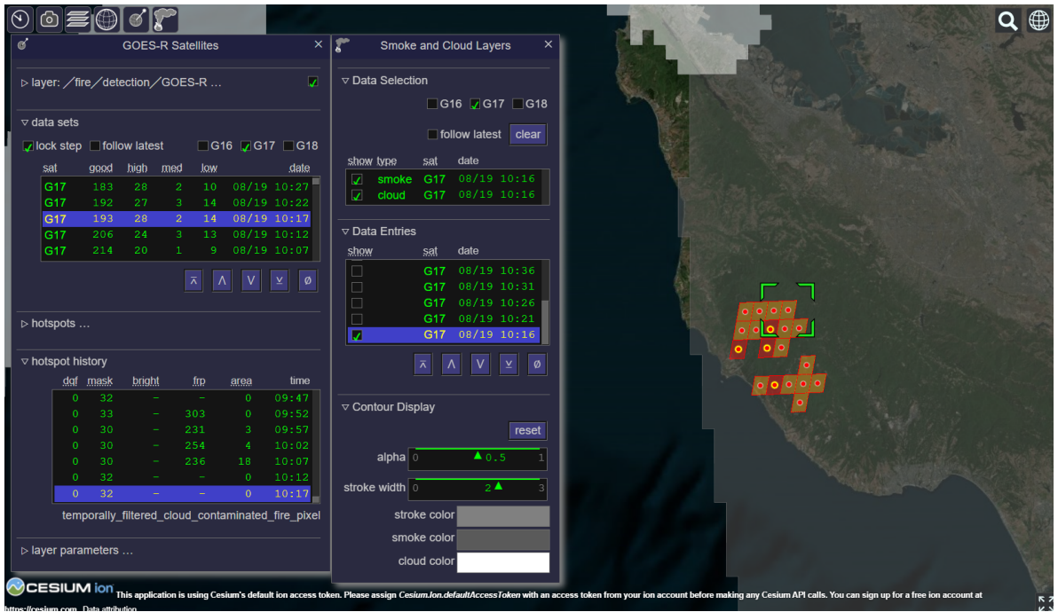
Figure 9: Smoke (grey pixels) and cloud (white pixels) segmentation and GOES-R hot spots in an ODIN application are shown with data from the CZU fire on August 19th, 2020 at 10:16 am.
