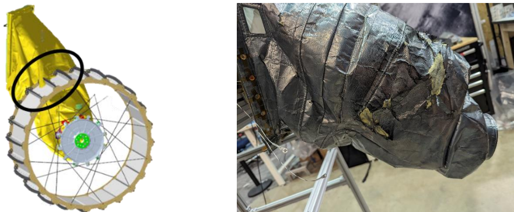
Figure V-4: Wheel-Sock interference region (left), and engineering development unit of Sock after wheel interference life testing.
