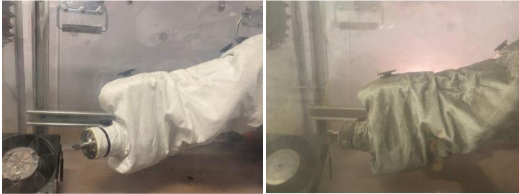
Figure V-2: Dust box test article before dust agitation (right) and after dust agitation (left)
