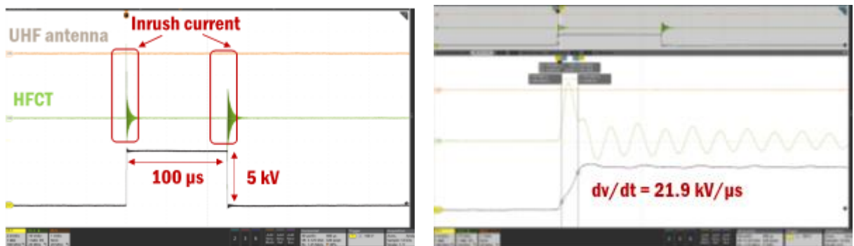
Figure 5-14. 5 kV, 100 \mu s pulse on DUT (left), and zoom on voltage edge (right)
