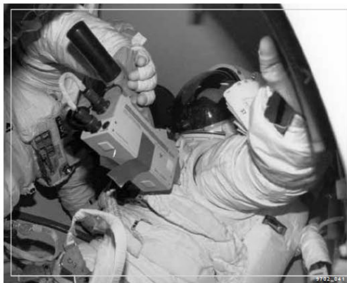
Figure 14-14. Compound-specific analyzer - hydrazine
