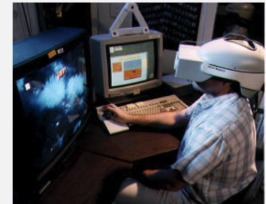
TROV telepresence interface operating underwater robot
