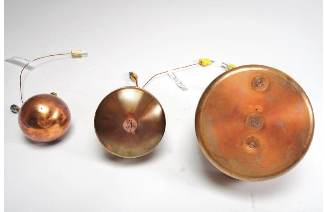
Representative slug calorimeters: 3 in hemisphere, 4 in iso-q, and 6 in flat
