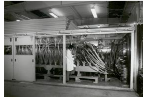
Interaction Heating Facility 60 MW - TPS Free Jet Testing
