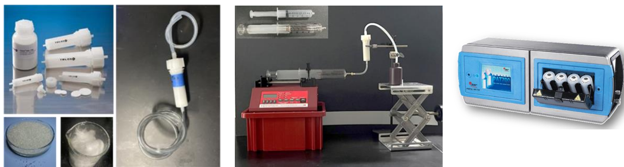
Figure 1. The first doser prototype: building material, test setup, and the TOC analyzer used for water analysis (shown from left to right).
