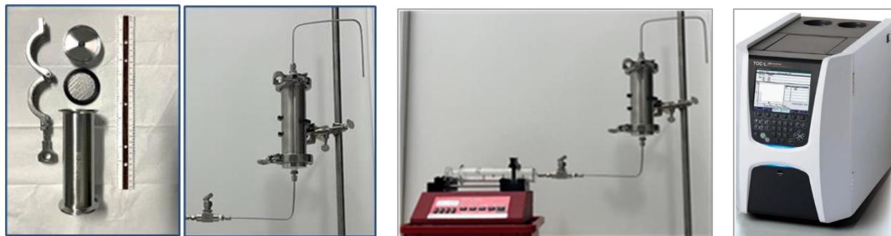
Figure 2. The second doser prototype: building material, test setup, and the TOC analyzer used for water analysis (shown from left to right).
