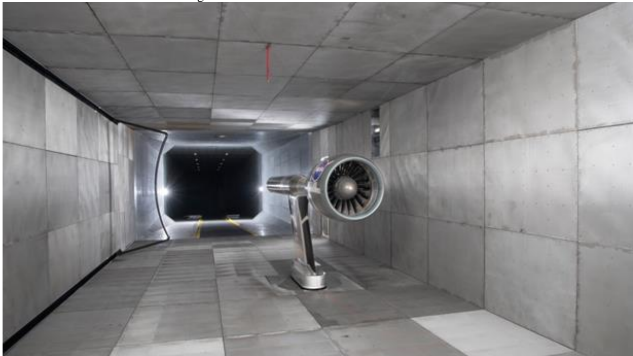
Figure 8 - NASA / P&W Advanced Ducted Propulsor in the 9×15 LSWT in 2022, acoustic configuration
